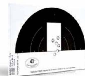
Six fast shots from both barrels in 9,3 x 74 R calibre. Note the even repartition of impacts.
