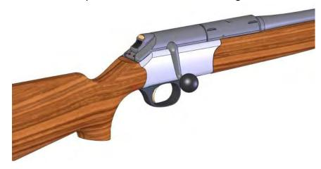
3) To de-cock your rifle, press the un-coking release button, located on top of the cocking device. A distinct "click" is heard then the cocking device slides rearwards, the 2 red dots are not showing anymore. The firing pin spring is now decompressed.
