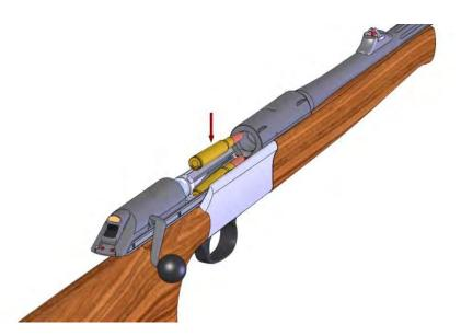
a) To empty your magazine, you are to remove it from the rifle. Once the magazine box in hand, eject the remaining cartridges by pushing them from back to front.
