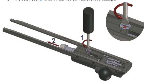
c. To insert a new bolt head, carefully selecting "Standard" or "Magnum" group, according to the letter "S" or "M" engraved on the extractor claw. Next, you are to insert the bolt head in its housing, while making sure that the firing pin is well positioned inside the new bolt head.
