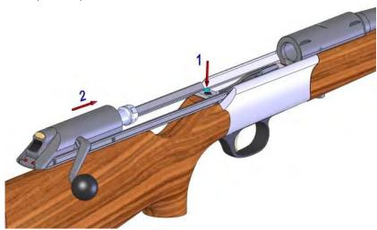
c) Push the bolt -3- with the bolt lever -4- until the bolt is locked into the barrel. Whenever these operations are not smooth, do not use extra strength, it simply means that the rails have not been correctly positioned on the receiver.
