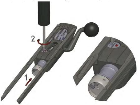
f. You can now insert the bolt assembly on the receiver. (Refer to § II-2)
