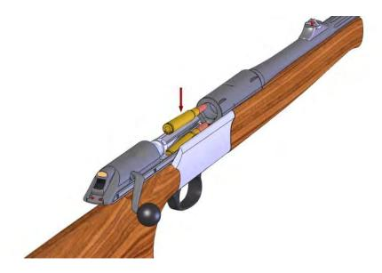
a) To empty your magazine, you are to remove it from the rifle. Once the magazine box in hand, eject the remaining cartridges by pushing them from back to front.
