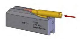
b) While hunting, you can shoot the first round, then open the bolt assembly and fill the magazine from the top, without taking it away from the receiver.
