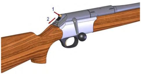
**WARNING** De-cocking the rifle automatically locks the bolt on the barrel. To re-open the bolt, you are first to cock the rifle. (Refer to § VI -1)
