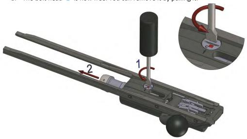
c. To insert a new bolt head, carefully selecting "Standard" or "Magnum" group, according to the letter "S" or "M" engraved on the extractor claw. Next, you are to insert the bolt head in its housing, while making sure that the firing pin is well positioned inside the new bolt head.
